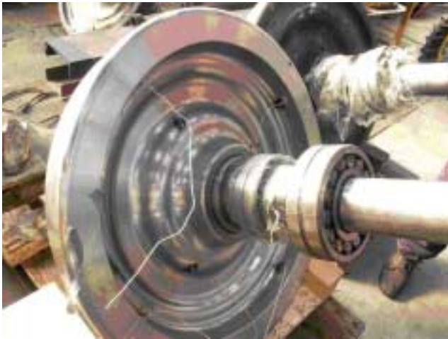
Fig. 14. Placing of thermocouples along the wheel circumference (9 mm away from the rolling surface)
