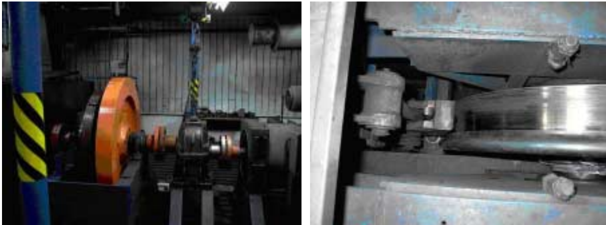
Fig. 12. Test stand for deformation and temperature investigation of railway wheelsets wheels
